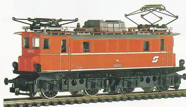
**115 10** Electric Bo'Bo' locomotive series 1040.10 of the ÖBB, hauling passenger and goods trains. Automatic light change, change over switch for overhead current supply.
