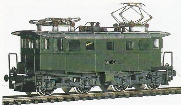
**113 00** Multi-purpose electric Bo'Bo' locomotive, series E 45 of the DR, change over switch for overhead current supply.
